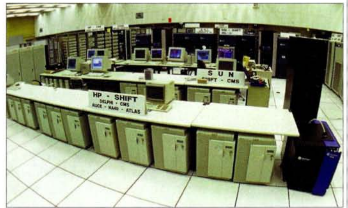
Ten years on: CERN's Computer Centre in 1998, with banks of SHIFT-distributed computing arrays for major experiments.
