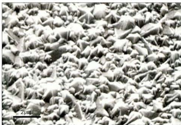
The polycrystalline growth of cubic boron nitride, which could replace diamond as the ultimate hard material.
