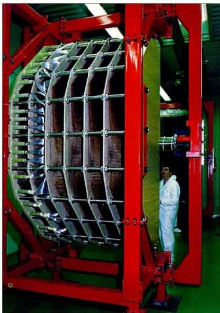
The support structure of the liquid-krypton calorimeter of the NA48 experiment at CERN. The calorimeter reconstructs the production of neutral pions, which is a key task en route to measuring the delicate CP violation in neutral kaon decays.
