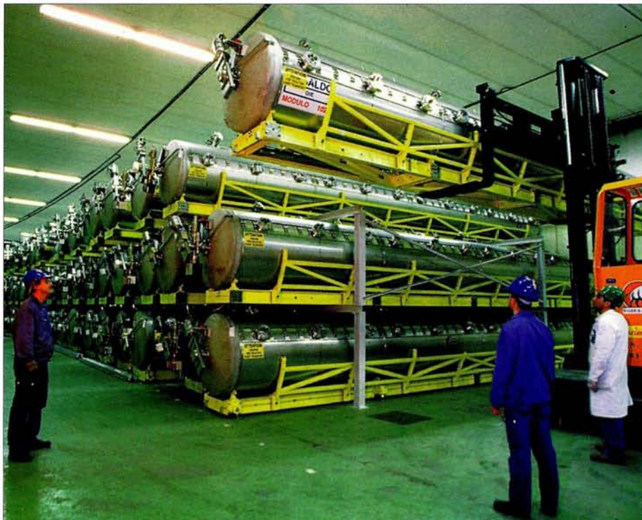
Superconducting radiofrequency equipment salvaged from CERN's LEP electron-positron collider could go on to be used in a new Superconducting Proton Linac.
